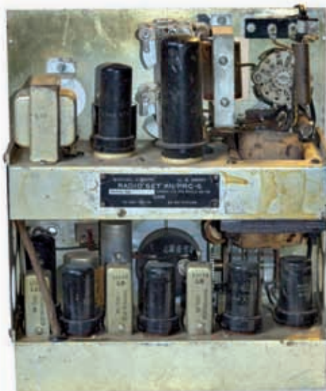
Fig. 5: Internal view of the PRC-5, transmitter on top, receiver below.
