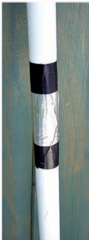
Fig. 2: A closer look at the foil capacitor on the antenna of Fig. 1.
