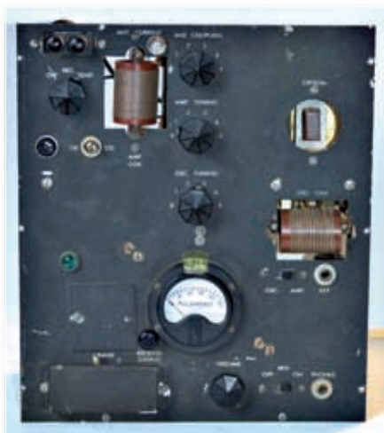
Fig. 4: The PRC-5 receiver transmitter, note the two coil units.
