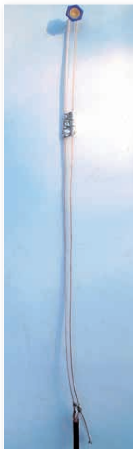
Fig. 3: A smaller ribbon cable antenna for u.h.f. work.
