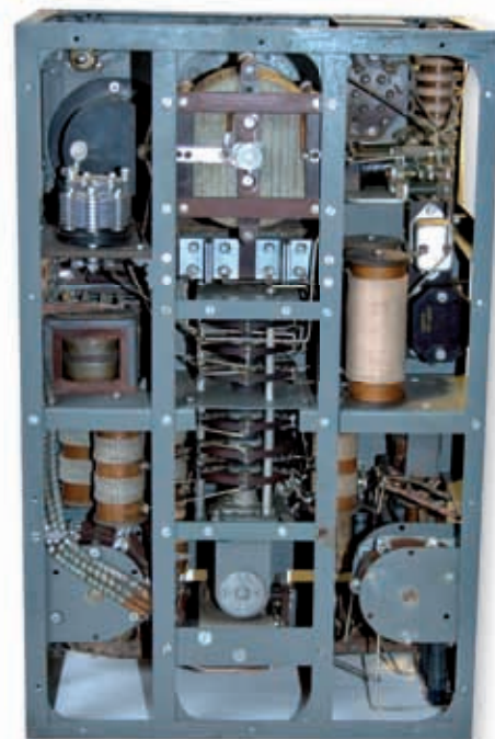
Fig. 2: Internal view of the Saram transmitter.
