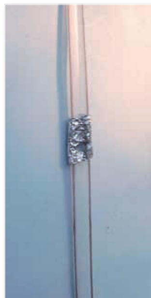
Fig. 4: a closer look at the tuning 'sleeve' capacitor of the antenna in Fig. 3.
